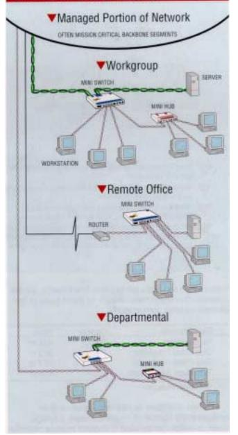
the remote office and the remote user the economy and flexibility of "pay as you go" telephone services. ISDN is a special telephone service that offers three channels, two 64 Kbps "B" channels for user data and a "D" channel for setting up the connection. With ISDN, the B channels can be combined for double the bandwidth or separated and used for different applications or users.
