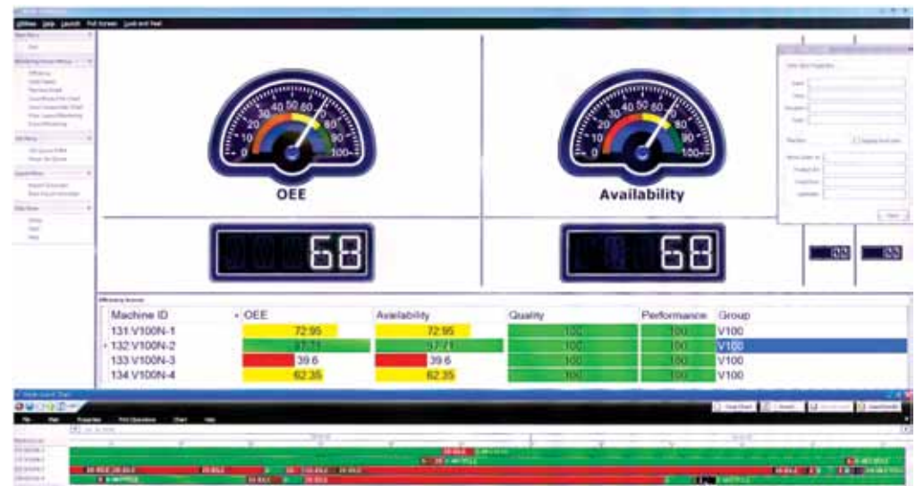
Mazak has adopted the MTConnect protocol, which incorporates the Memex Merlin monitoring software. The system has been integrated into Mazak's iSmart factory concept.
