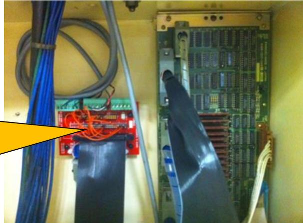
Orange jumper wires on the Ax650 board allow a quick selection of any of the 50 conductors located on the Honda connector, routed to a point on one of the green supplied Phoenix connectors
