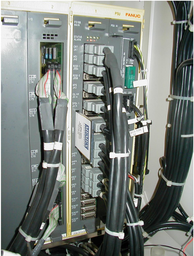
Fanuc 16MB with PCMCIA SRAM in the MEM card slot on the A16B-3200-0010 CPU card.
