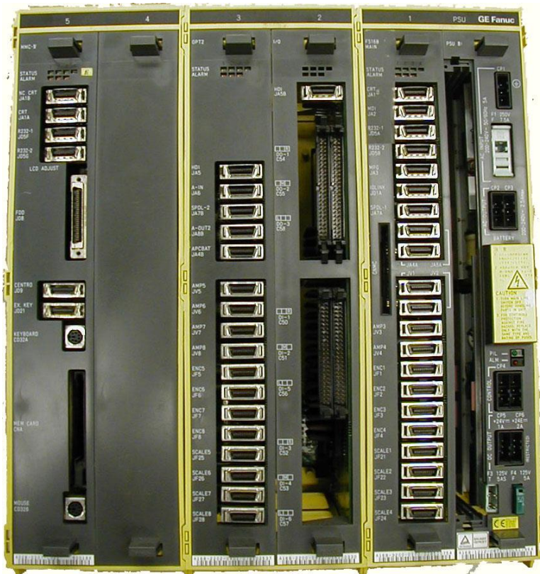
Fanuc 16B Control CPU Card (0010 CPU Card is 2 nd from right in this picture beside the power supply)
